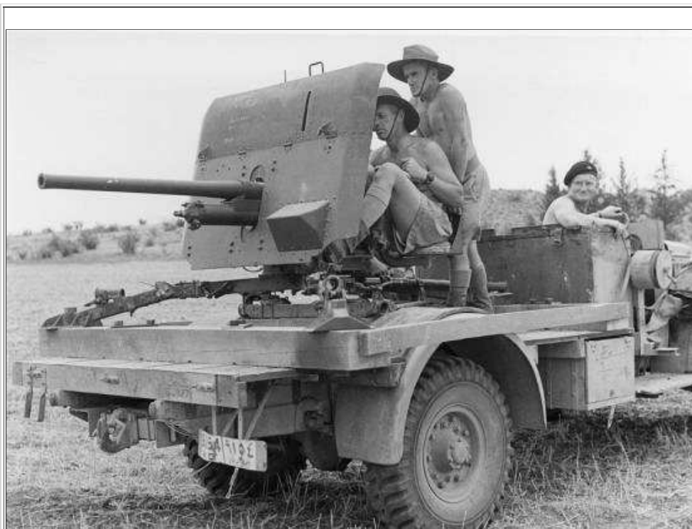
A towed 2 Pounder Anti-tank Gun with wheels removed and mounted on the back of a Morris CS 11 30 Cwt 4x2 truck. The truck body has been removed and a wooden frame built to carry the legs of the gun's ground mount. Note the variety of headdress.
